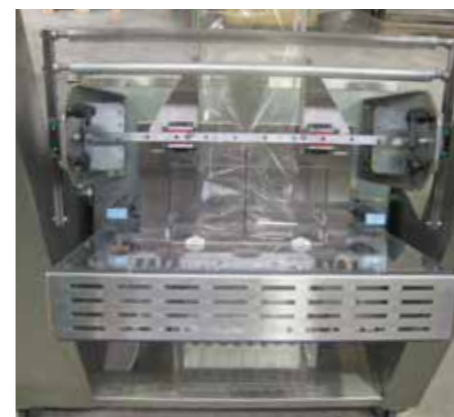
Inclinable working level from 0° to 90°.
