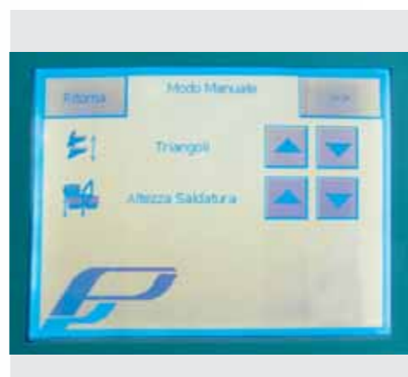
Easy change of format: center sealing and triangle-inverting head motorised. Height up 400 mm.
