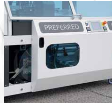
Film dispenser unit and film wind up unit both in front of the machine easy to be reached. Remarkable user-friendliness .Sliding door.
