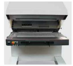
Opening chamber available for cleaing and maintenance.
