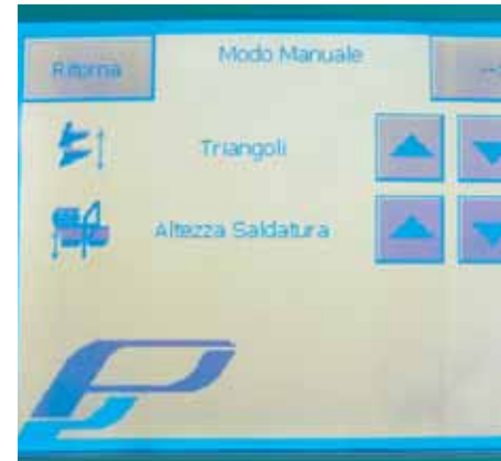
Easy change of format: center sealing and triangle-inverting head motorized. Height up 400 mm.
